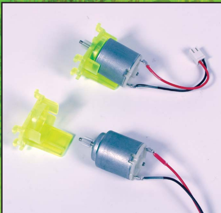
FIGURE 5. Mount the left and right drive motors in their respective motor mounting plate. Both mounting plates are the same, there is no assigned left or right plate.
